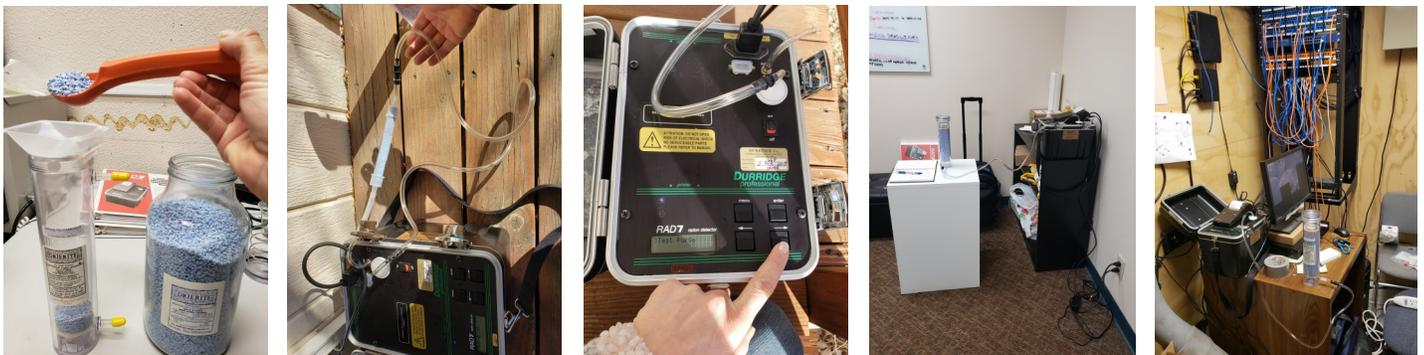
*Pictures from left: Desiccant is used to reduce humidity in incoming sample air and for a "dry purge" of the ion chamber in the detector; a regular purge cycle is performed between sampling runs; sampler set up to run at Tribal Headquarters; set up at Head Start.*
